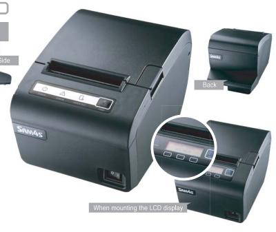
ELLIX 30/40 have been made as a modern and compact design to meet customers' diverse needs and are new era receipt printers with powerful printing capabilities and various additional functions.
