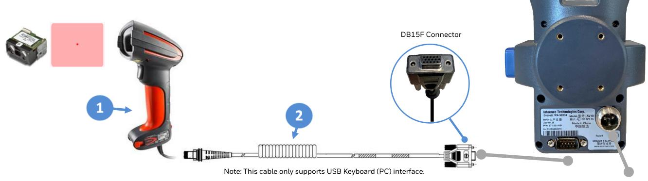
Note: Vehicle Dock must have external power connected for DB15 USB port to be active.
